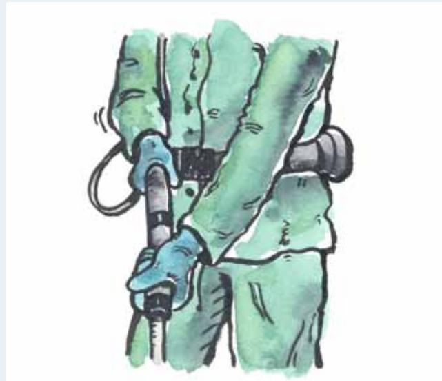
Support the elbow of the arm with which you steer the lance (here it is the right arm). Your shoulder and elbow joints will be least stressed in that way.
